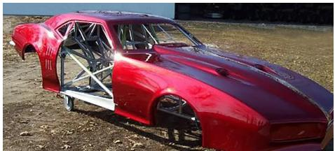
**CDRC Top Sportsman Chassis Roller Package** features a CDRC 4130 Moly 25.1E Advance ET Chassis with CDRC Fabricated 9" 4130 Moly Housing with specialized chassis design for your horsepower combination.
